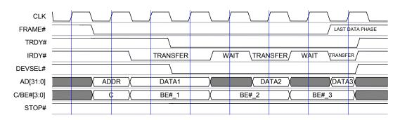
Figure 6.20: PCI Initiator to Target Burst Write cycle
