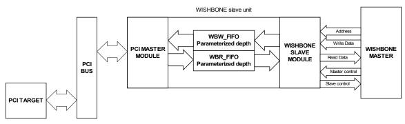
Figure 3.4: WISHBONE Slave Unit Architecture Overview
