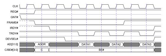
Figure 6.7: PCI Burst Read Cycle
