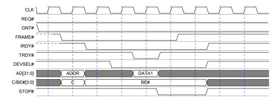
Figure 6.13: Target Disconnect without data
