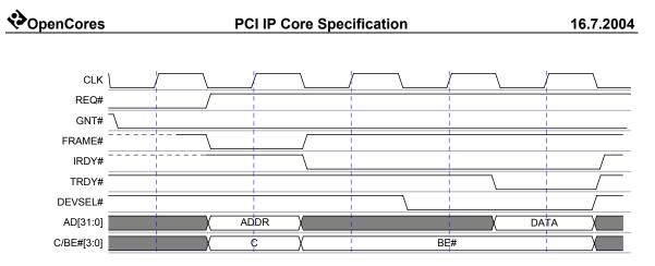
Figure 6.5: PCI Single Read cycle
