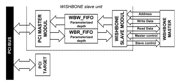
Figure 2.2: WISHBONE slave unit architecture
