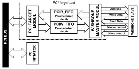
Figure 2.3: PCI target unit architecture overview
