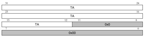
Figure 4.11: PCI Translation Address register layout
