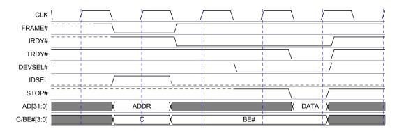
Figure 6.15: PCI Configuration Read cycle
