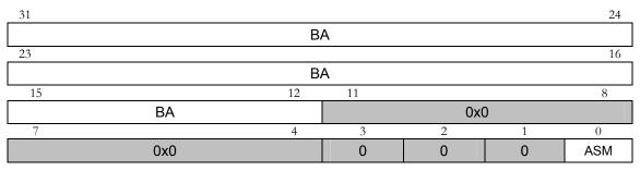
Figure 4.9: PCI Base Address Register Layout
