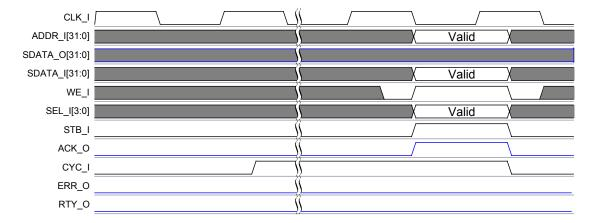
Figure 6.2: WISHBONE Configuration Write cycle
