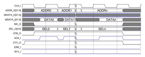
Figure 6.18: PCI to WISHBONE Read cycle
