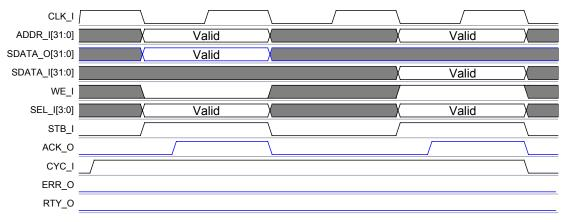
Figure 6.3: WISHBONE configuration RMW cycle
