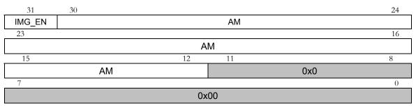
Figure 4.10: PCI Address Mask register layout
