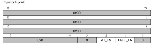
Figure 4.8: PCI Image Control register layout
