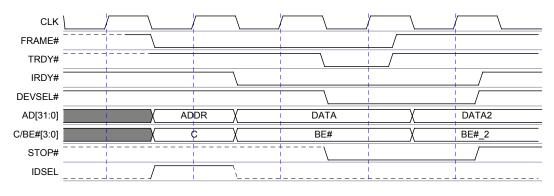
Figure 6.16: PCI Configuration Write cycle
