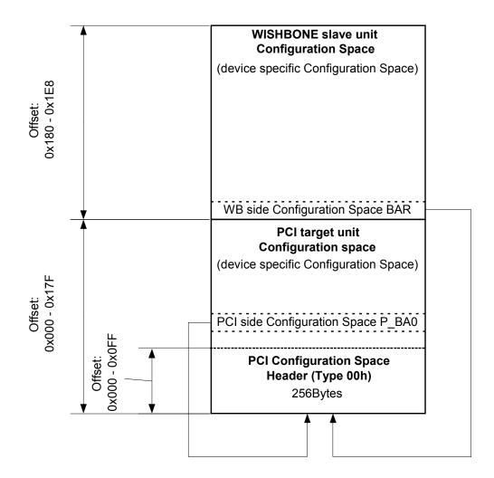
Figure 3.1: PCI Bridge Configuration Space
