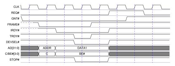
Figure 6.14: Target Disconnect with data
