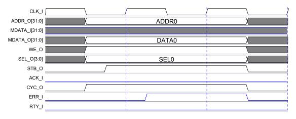
Figure 6.23: Error on WISHBONE bus caused by PCI to WISHBONE transfer
