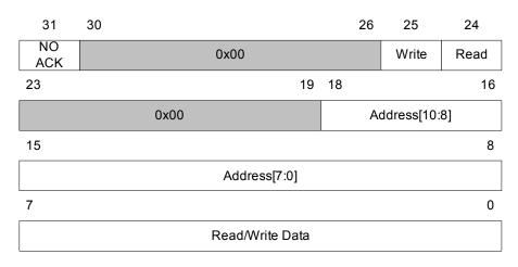
Figure 3.8: 3.9.3. Serial EPROM Control and Status Register layout
