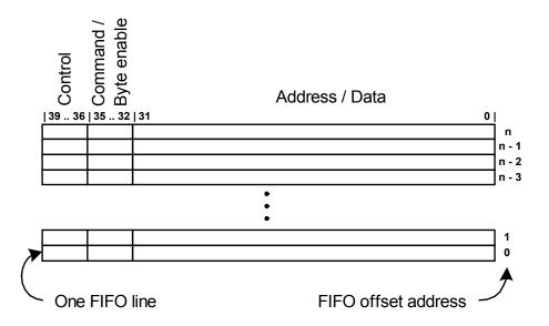
Figure 2.4: Detailed Description of FIFO Register Lines
