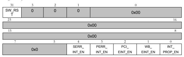
Figure 4.15: Interrupt Control register layout
