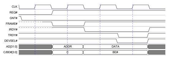
Figure 6.6: PCI Single Write
