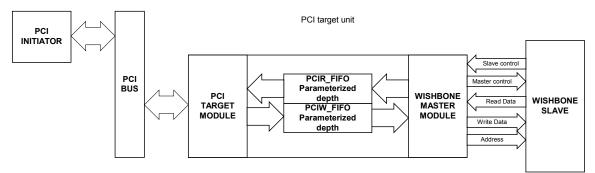
Figure 3.5: PCI target unit architecture overview
