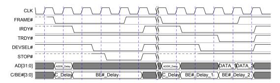
Figure 6.17: PCI Target Read cycle
