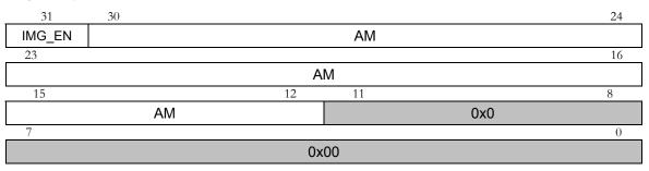
Figure 4.4: WISHBONE Address Mask register layout
