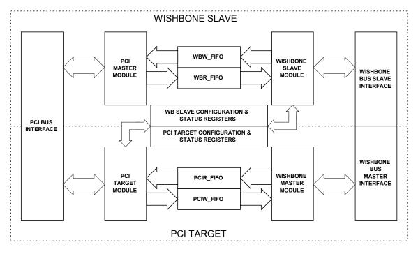
Figure 2.1: PCI bridge core architecture
