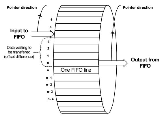
Figure 2.5: FIFO Architecture
