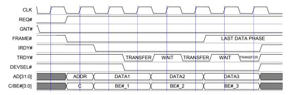
Figure 6.8: PCI Burst Write cycle
