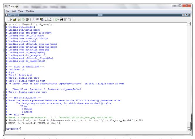
The transcript window clearly shows points in time where the simulation starts, ends, and where errors are detected. The simulation stops with a clear SUCCESS/FAIL message, specifically formatted for parsing by scripts.
