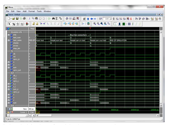
During a simulation, the waveform window shows current test number, test name, user-defined info, accumulated number och checks and errors. When the error counter increments, a bug has been found in that point in time.
