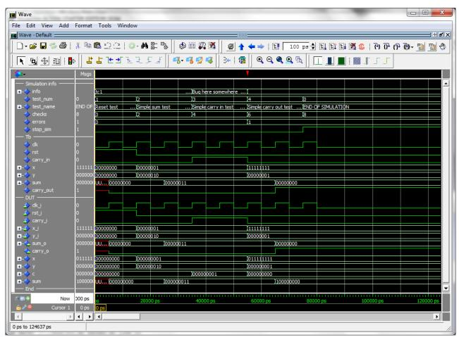
Here we can see the error detected at the point in time when the error counter increments. Again, we can that the error is found in test 3, the Simple carry in test.
