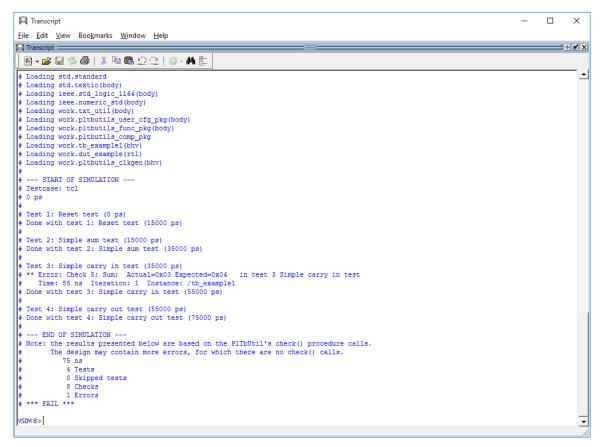
The transcript window clearly shows points in time where the simulation starts, ends, and where errors are detected. The simulation stops with a clear SUCCESS/FAIL message, specifically formatted for parsing by scripts.
