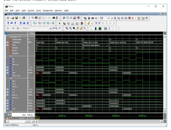
Here we can see the error detected at the point in time where the error counter increments from 0 to 1. Again, we can that the error is found in test 3, the Simple carry in test.
