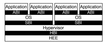
Figure 1.1: Different implementation stacks supporting various forms of privileged execution.
