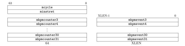
Figure 3.16: Hardware performance monitor counters.
