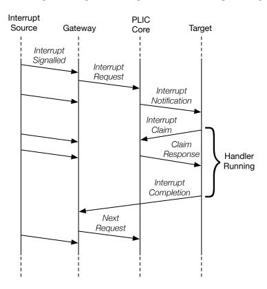
Figure 7.2: Flow of interrupt processing via the PLIC.
