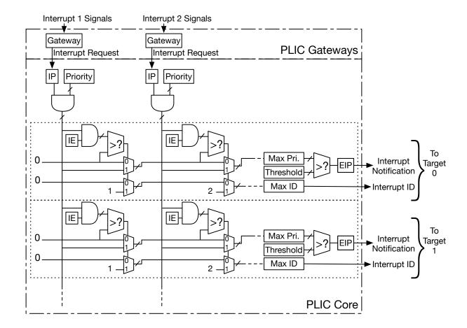
Figure 7.1: Platform-Level Interrupt Controller (PLIC) conceptual block diagram. The figure shows the first two of potentially many interrupt sources, and the first two of potentially many interrupt targets. The figure is just intended to show the logic of the PLIC's operation, not to represent a realistic implementation strategy.
