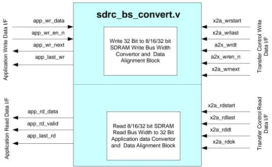
During write transaction, it split the 32 Bit Application data into 8/16/32 SDRAM Bus width format.
