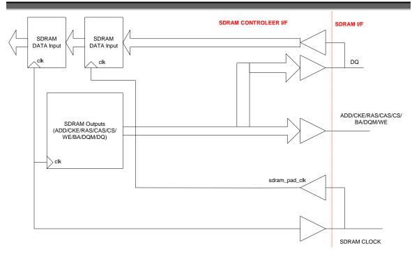
To simply the interface timing issue at SDRAM interface, all the output signals are driven with SDRAM\_CLOCK. DQ Input is captured with Delayed sdram\_pad\_clk.
