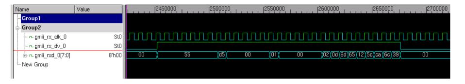
The above waveform shows a sample packet reception. RX\_DV is asserted for the entire time the packet is transmitted, and the low to high transition on RX\_DV indicates start of transmission.
