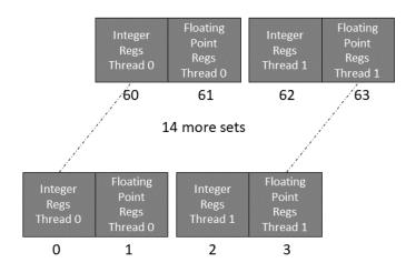
On reset register set #0 is selected to be the operating register set. On interrupt every fourth register sets #4 to #28 will be selected according to the level of the interrupt.
