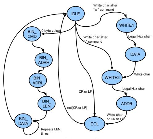
Figure 2: Parser State Diagram
