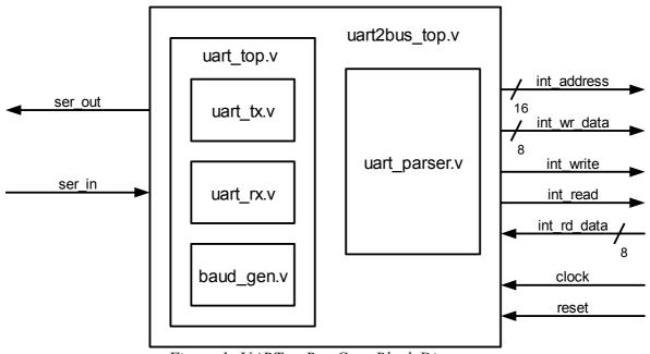
Figure 1: UART to Bus Core Block Diagram
