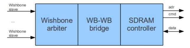
Asynchronous design where wishbone and SDRAM clock domain are independant. Multiple wishbone port with use of a wishbone arbiter.
