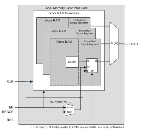
Figure 67: Virtex-5 FPGA Block Memory Generated with Register Port [A|B] Output of Memory Primitives Enabled
