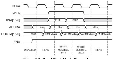
Figure 27: Read First Mode Example
