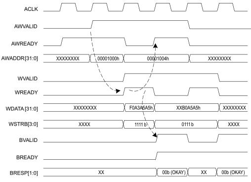
Figure 9: AXI4-Lite Single Burst Write Transactions
