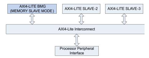
Figure 4: AXI4-Lite Memory Slave Application Diagram
