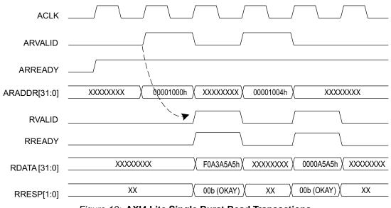
Figure 10: AXI4 Lite Single Burst Read Transactions
