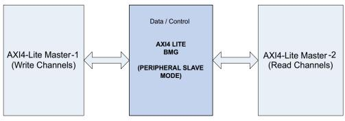
Figure 8: AXI4-Lite Peripheral Slave Application Diagram
