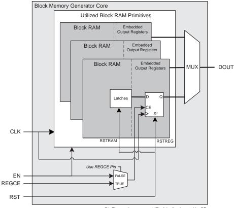
$\mathsf{S}^\star$  : The synchronous reset (S) of the flop is gated by CE
