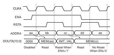
Figure 39: Reset Behavior When Reset Priority is Set to CE
