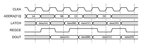
Figure 38: Flow Control Using REGCE
