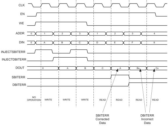
Figure 47 shows the assertion of the SBITERR and DBITERR output signals when errors are injected through the error injection pins during a Write operation.
