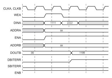
*Figure 46:* Read and Write Operation with BuiltIn\_ECC in Zynq-7000, 7 Series, Virtex-6, and Virtex-5 FPGAs
