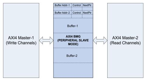
Figure 5: AXI4 Peripheral Slave Application Diagram
