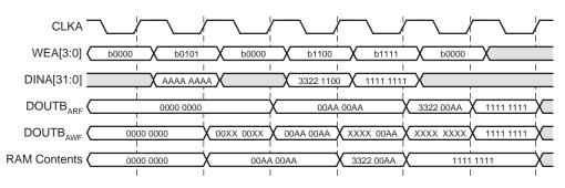
Figure 33: Write-Read Collision Example
