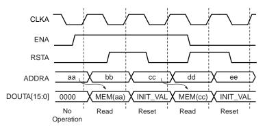
Figure 40: Reset Behavior When Reset Priority is Set to SR
