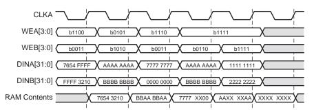
Figure 32: Write-Write Collision Example
