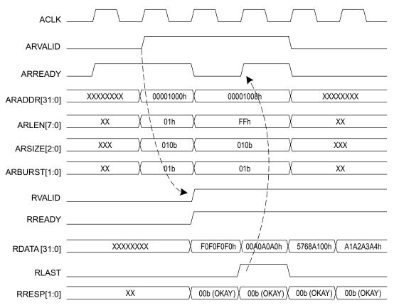
Figure 12: AXI4 Incremental Read Burst Transactions
