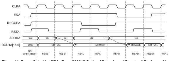
Figure 44: Reset Gated by CE in Zynq-7000, 7 Series, Virtex-6, and Spartan-6 Devices with Reset Memory Latch Option
