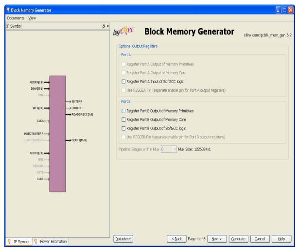
Figure 50: GUI Page 3: Enabling Input/Output Registering Stages
