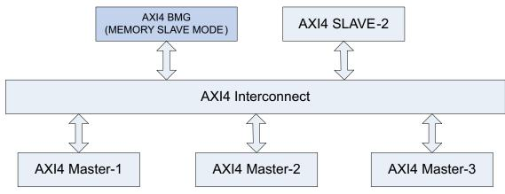
Figure 3: AXI4 Memory Slave Application Diagram
