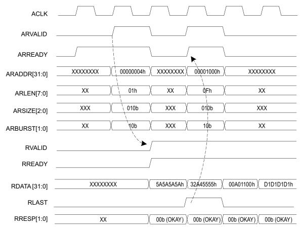
Figure 14 illustrates the timing on AXI WRAP or cache line burst Read transactions.
