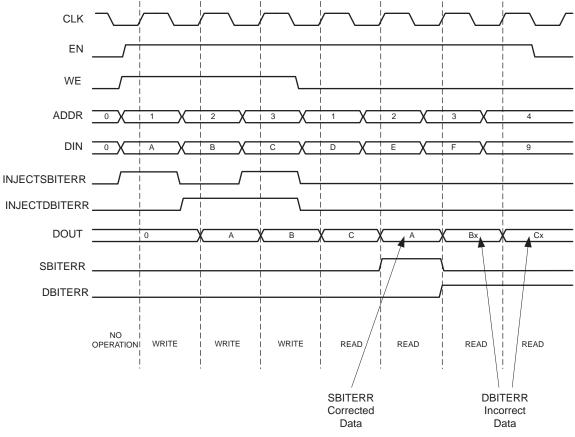
Figure 52: Assertion of SBITERR and DBITERR Signals
