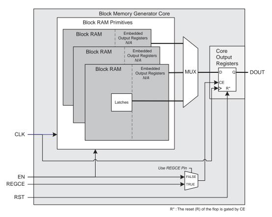
Figure 70: Zyng-7000, 7 Series, Virtex-6, Virtex-5, or Virtex-4 Block Memory Generated with Register Port [A|B] Output of Memory Core Enabled
