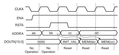
Figure 41: Standard Reset Behavior Similar to Previous Architectures
