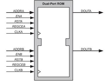
The Dual-port ROM allows Read access to the memory space through two ports, as shown in Figure 19.
