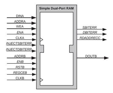
*Note:* For Virtex family architectures, Read access is via port A and Write access is via port B.
