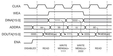
Figure 26: Write First Mode Example
