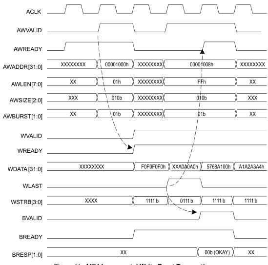
Figure 11: AXI4 Incremental Write Burst Transactions
