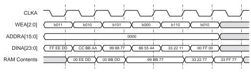
Figure 31: Byte-Write Example
