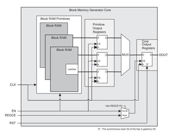
Figure 34: Spartan-3 Block Memory: Register Port [A|B] Outputs of Memory Primitives and Memory Core Options Enabled
