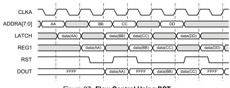
Figure 37: Flow Control Using RST
