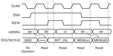
Figure 45: Asynchronous Reset
