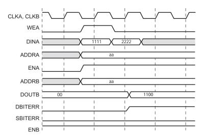
Figure 51: Read and Write Operations with Soft ECC
