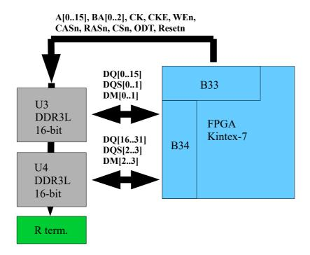
Two currently available FPGA variants enable max. data rates 667 Mb/s (-1FBG676C) or 1066 Mb/s (-2FFG676C) provided DDR3L (1.35V) memory chips are used. Higher data rates of 800 Mb/s respectively 1333 Mb/s are achievable with DDR3(1.5V) devices.
